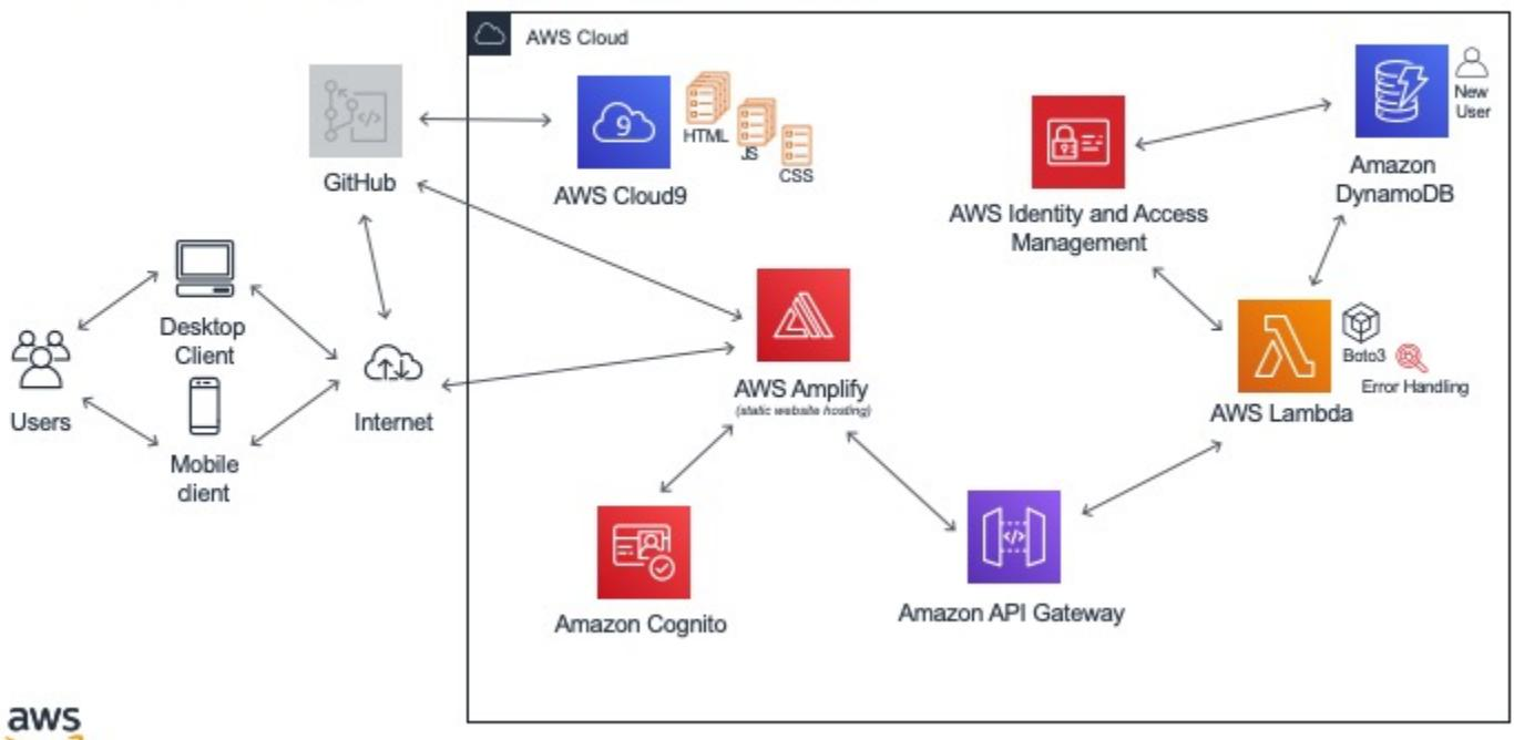
The next step we need to be able to do is create a new row in the database. To do this we run the command **put\_Item**. We will once again have to make a Lambda function to run this code. We will not actually create an API Gateway to access this code, instead in the next step we will get Cognito to automatically **trigger** this Lambda function when a new user is created.
