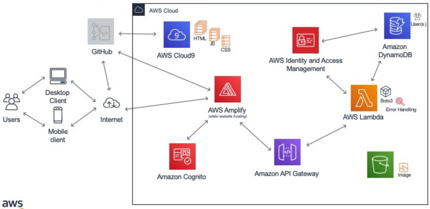
A next nice step would be if we could upload an image to use as the profile image of the user. The problem is that an image cannot be saved into our DynamoDB table. It can only hold text or numbers. What we can do instead is create an S3 bucket and save our images into it. Then we just save the key in our table, that points to our particular image.
